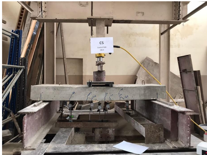
Fig. (4) – “CS” Control slab cracks shape
