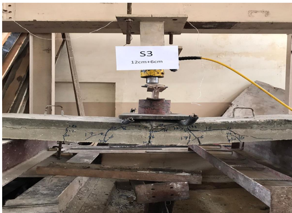
Fig. (7) – “S3” Slab 3 cracks shape
