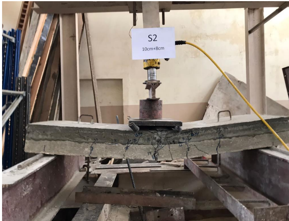
Fig. (6) – “S2” Slab 2 cracks shape
